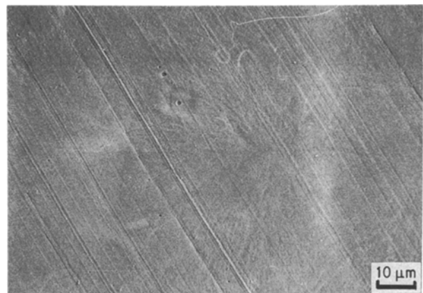
Figure 4 SEM micrographs of vacuum moulded PPI, 45° tilt.
